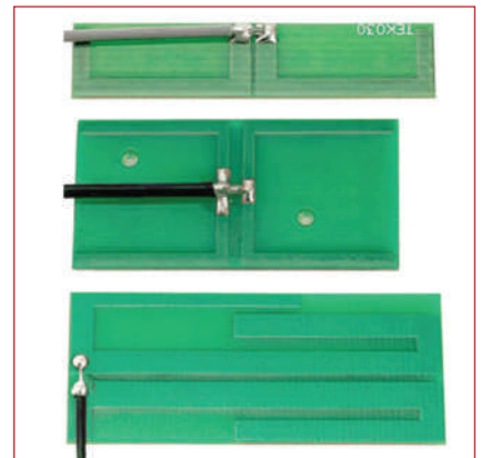
▲ Fig. 6 Dipole antennas using bent conductive elements to save space.
